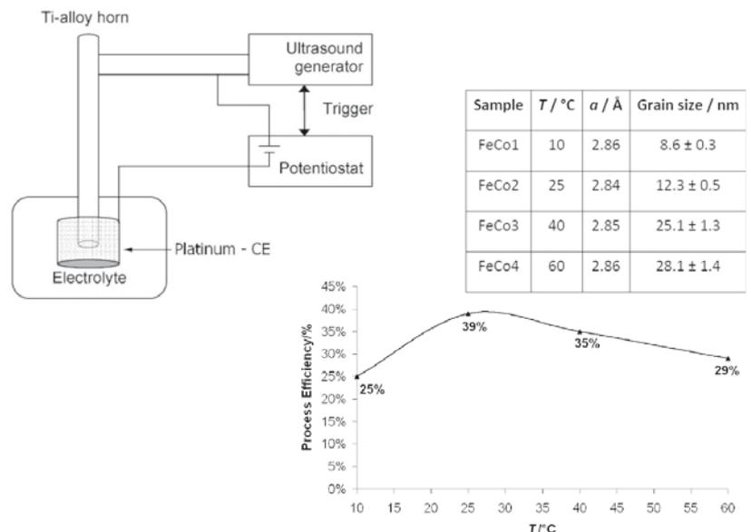
Fig.2. Effect of bath's temperature on final process efficiency
