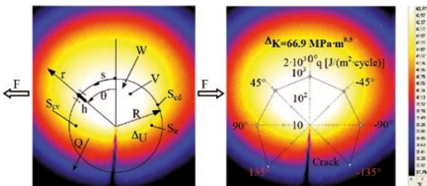
**Fig.1. Energy balance for a volume of material  $V$  surrounding a crack tip subject to Mode I fatigue loadings.**
