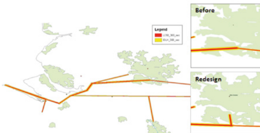
Figure 2 Pipeline network near Manchester city: CO 2 consequences due to full bore rupture and redesign network to improvement the safety near center of city.
